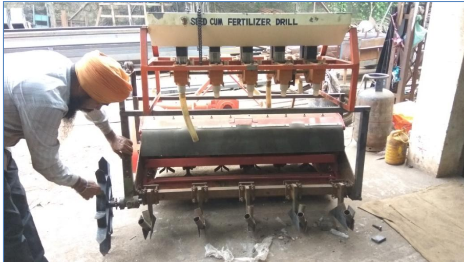
Fabrication of a seed cum fertilizer metering assembly with roller & cup type metering mechanism and fitting with straw chopper
