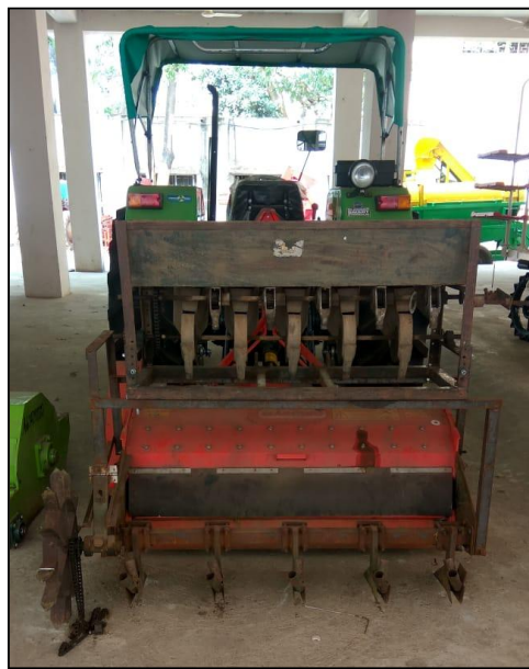
Fabrication seed cum fertilizer delivery assembly with fluted roller metering mechanism and fitting with Straw chopper cum seeder
