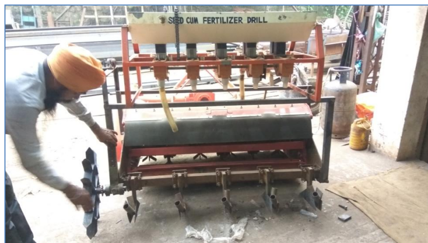
Fabrication of furrow opening assembly with five nos zero till tynes and fitting with straw chopper
