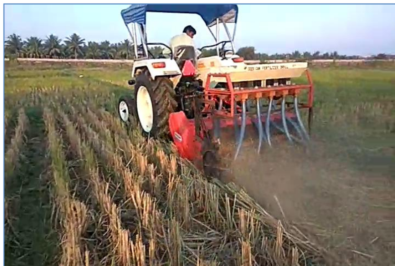
Performance evaluation of the developed straw chopper cum seeder in OUAT research station
