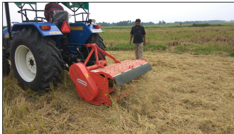
Evaluation of the tractor operated straw chopper in OUAT Research Station
